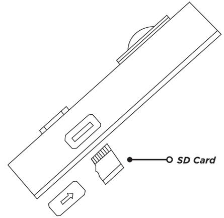
Figure 7: Installing the SD Card
