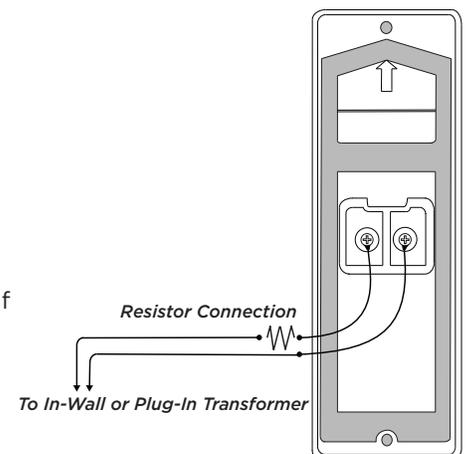
Figure 5: Resistor Connection to in-wall or plug-in transformer
