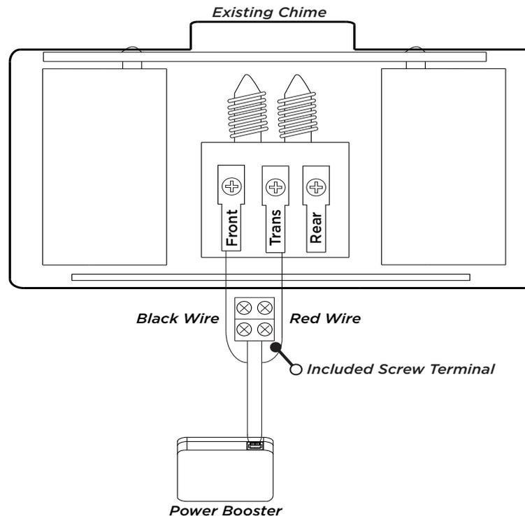
Figure 4: Installing the Power Kit
