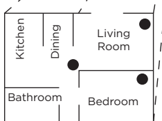
Figure 9: Smoke Detector Placement Locations
