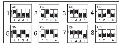
**Figure 2: Supervised keypad addresses**
