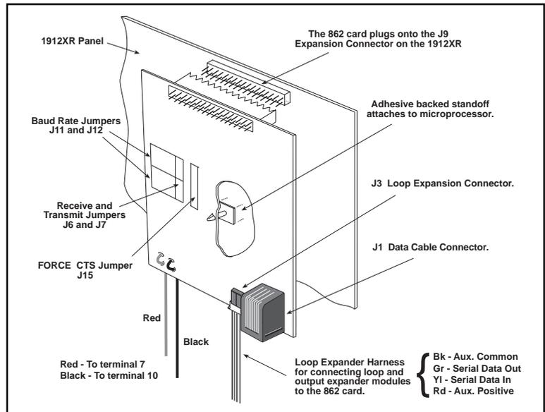
Figure 1: Installing the 862 on the 1912XR panel
