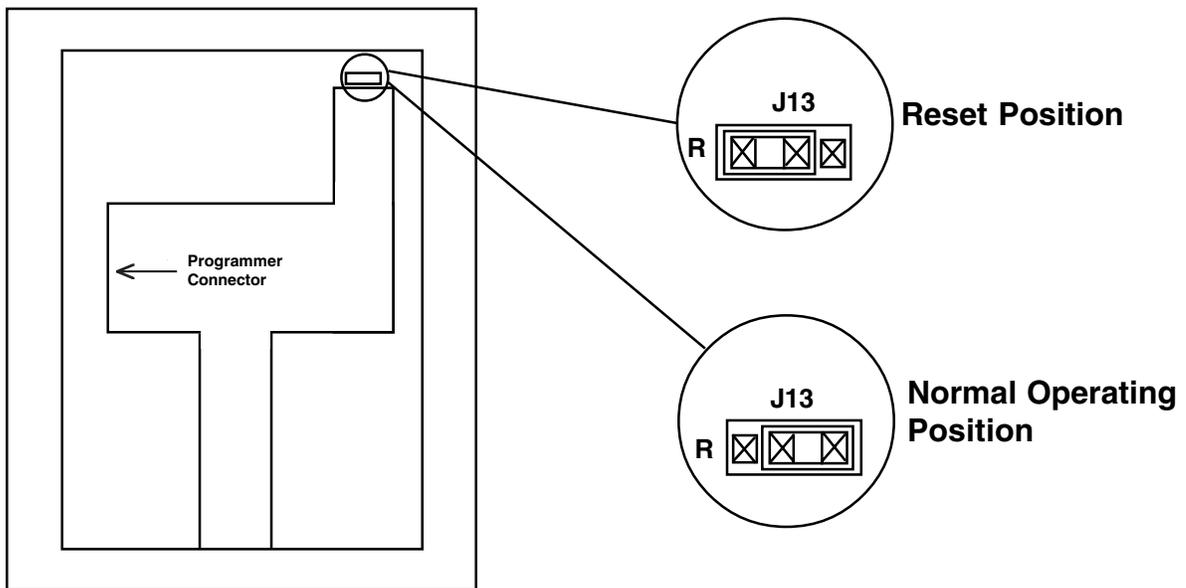
After the programmer is installed move J13 to the right hand position to start the programmer. Programming is done from SECURITY COMMAND address number 1. To remove the programmer, first place J13 in the reset position, then remove the programmer. Always place J13 in the reset position when installing or removing the programmer.
